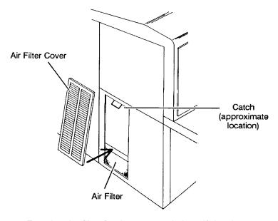
2. Examine the filter for dust accumulation. If dust has accumulated, follow the instructions in the *Replacement Procedures*.
